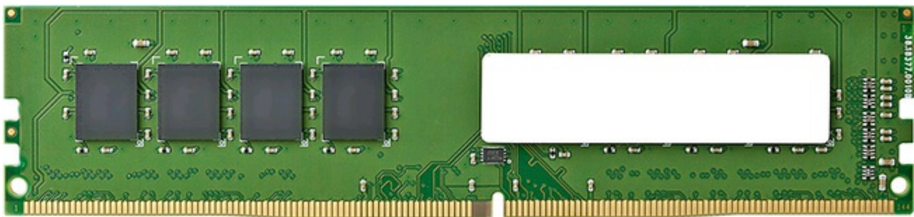
FIGURE 6.5 A typical 8GB DDR4 module without heat spreaders.
