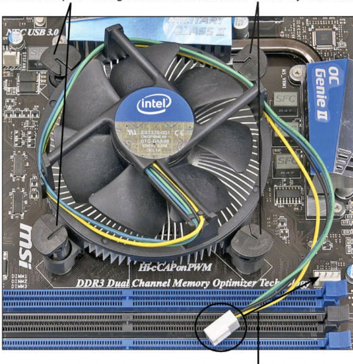
FIGURE 18.10 An Intel heatsink being installed on an LGA1155 processor.
