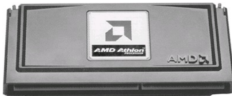
FIGURE 3.35 AMD Athlon processor for Slot A (cartridge form factor).
