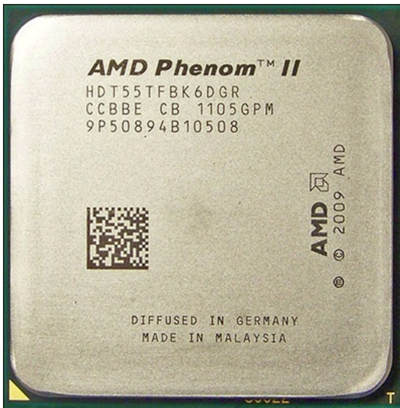
FIGURE 3.40 The Phenom II X6 conceals six cores and memory controllers for both DDR2 and DDR3 memory beneath its protective metal spreader plate.
