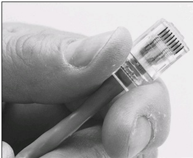
FIGURE 16.12 Push the 8P8C (RJ-45) connector into place, ensuring the cable pairs are ordered properly.
