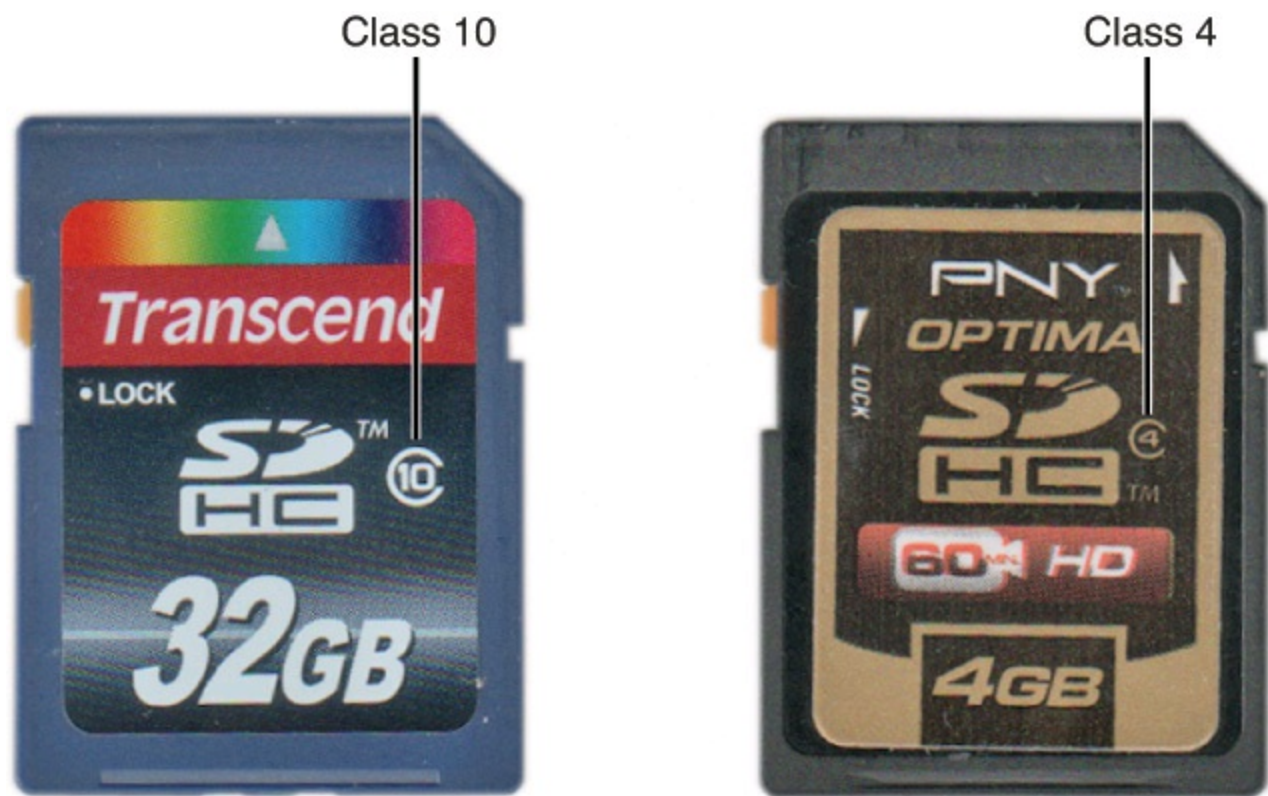
FIGURE 9.5 Speed class markings on typical SDHC cards.
