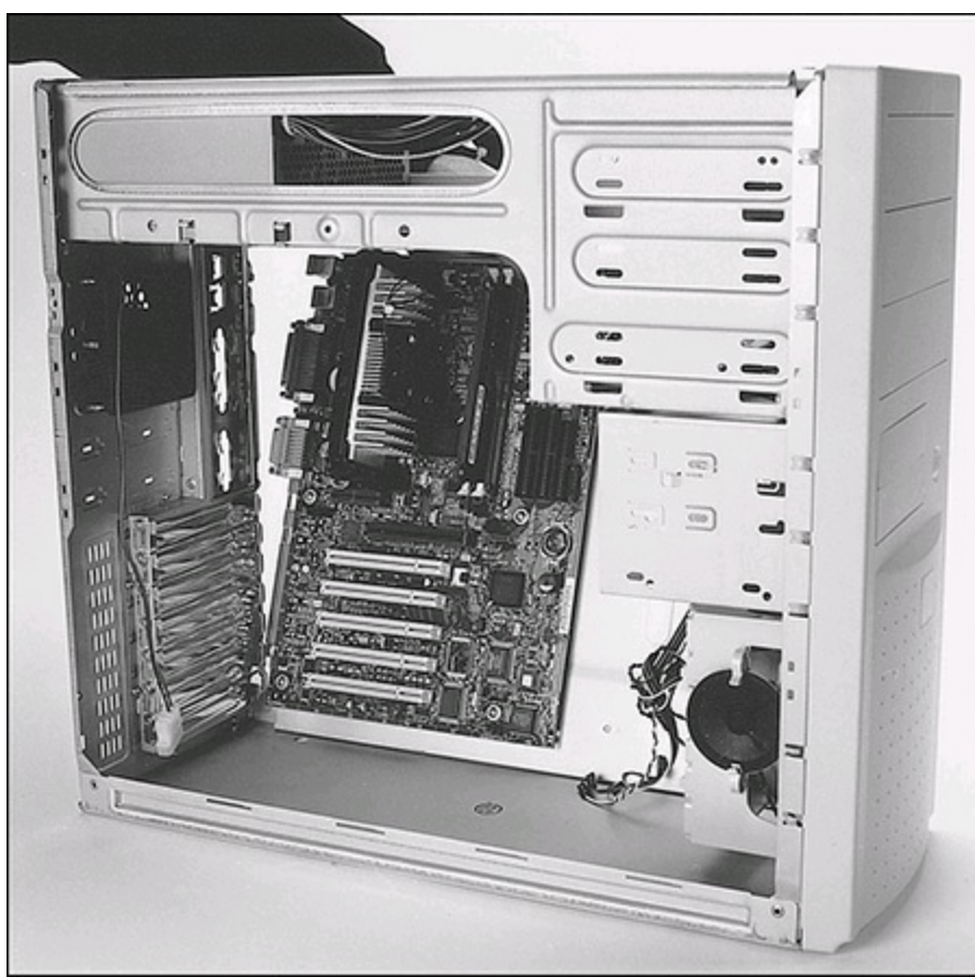
FIGURE 18.20 Installing a motherboard and tray into the chassis.
