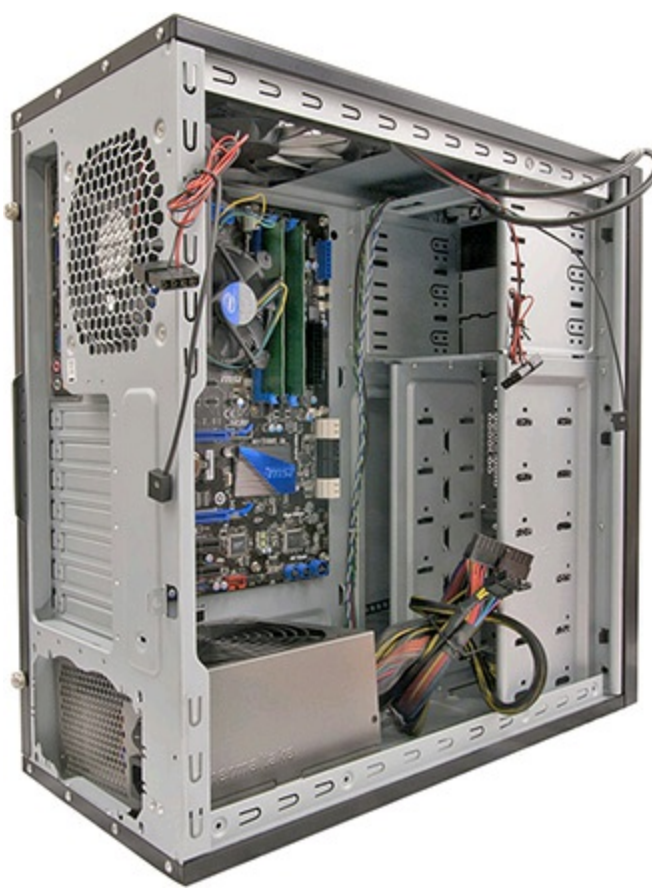
FIGURE 18.23 Installing the power supply into the chassis.
