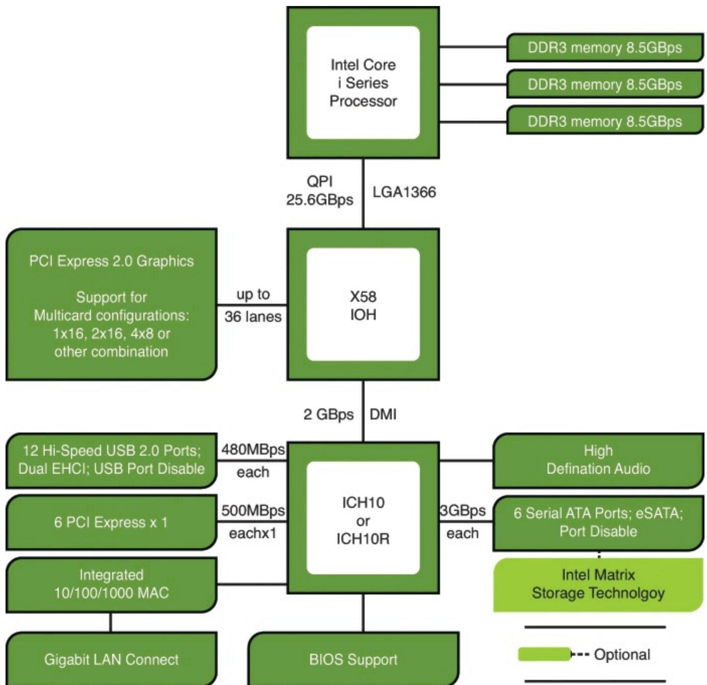
FIGURE 4.23 Block diagram of a system with a socket LGA1366 Core i-series processor and an X58 Express chipset.
