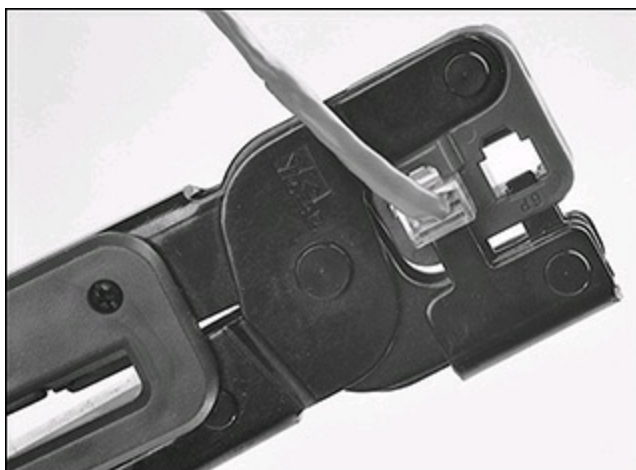
FIGURE 16.13 Firmly squeeze the crimping tool to attach the connector to the cable.
