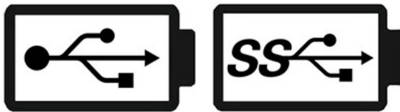
FIGURE 13.16 Typical identification marks for USB 2.0 (left) and USB 3.0/3.1 (right) Power Delivery cables.
