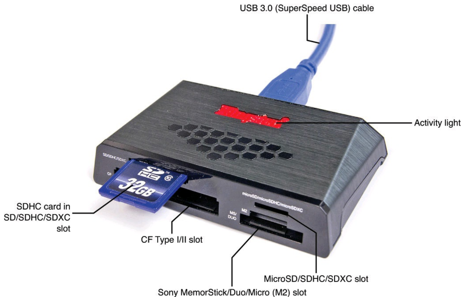
FIGURE 9.6 The Kingston FCR-HS3 card reader plugs into a USB 3.0 (or USB 2.0) port and assigns a drive letter to each slot for easy copying of files between cards.
