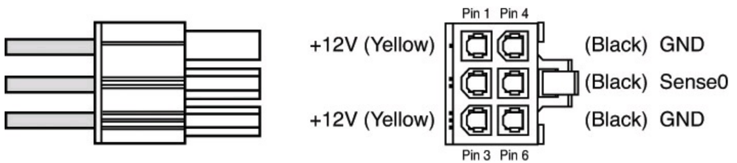
FIGURE 17.34 PCI Express 6-pin (2×3) auxiliary 75W power supply connector.
