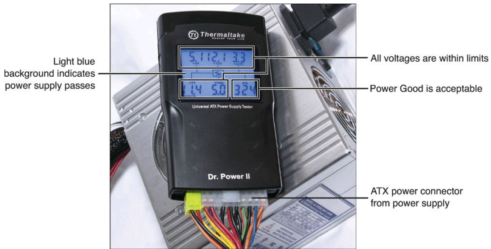
FIGURE 17.41 This power supply works and provides correct voltage levels.
