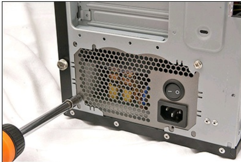
FIGURE 18.24 Installing the screws to retain the power supply.
