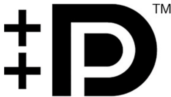
FIGURE 11.18 Icon indicating a DisplayPort with Multimode (DVI and HDMI) support.
