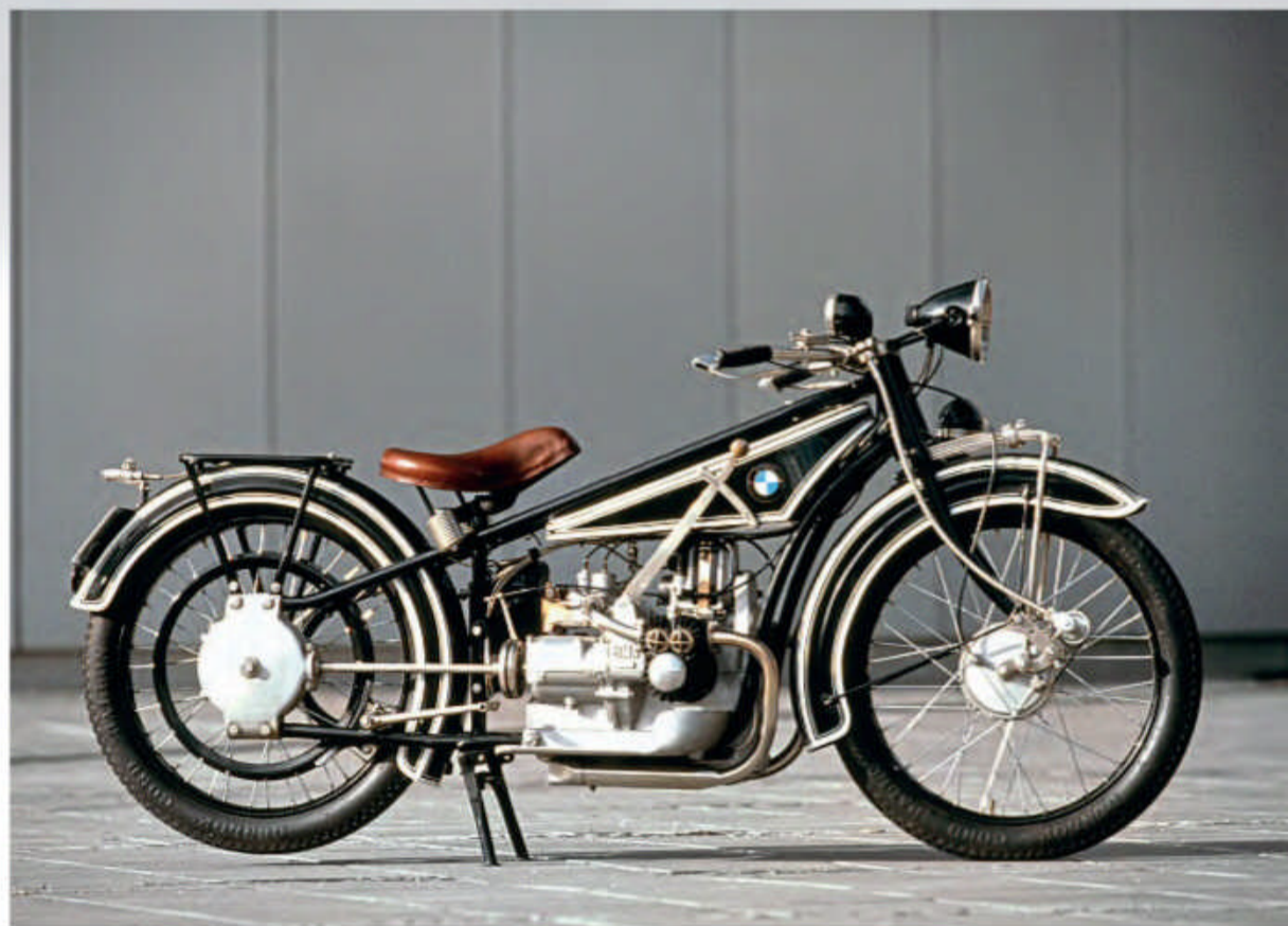
An early example of Germany’s BMW, with the boxer engine.
