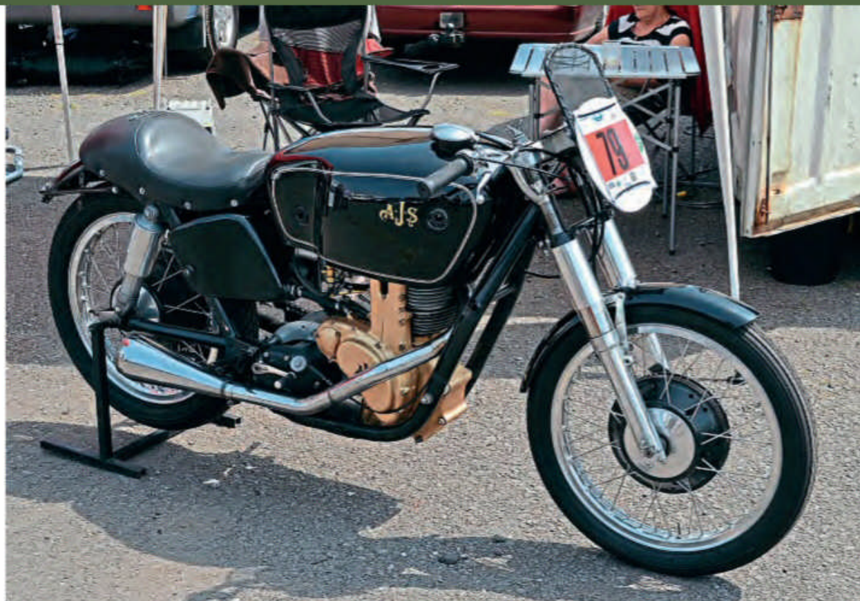
The AJS 7R, with its gold-finished engine and black paintwork, cut quite a dash. This is a long stroke version.
