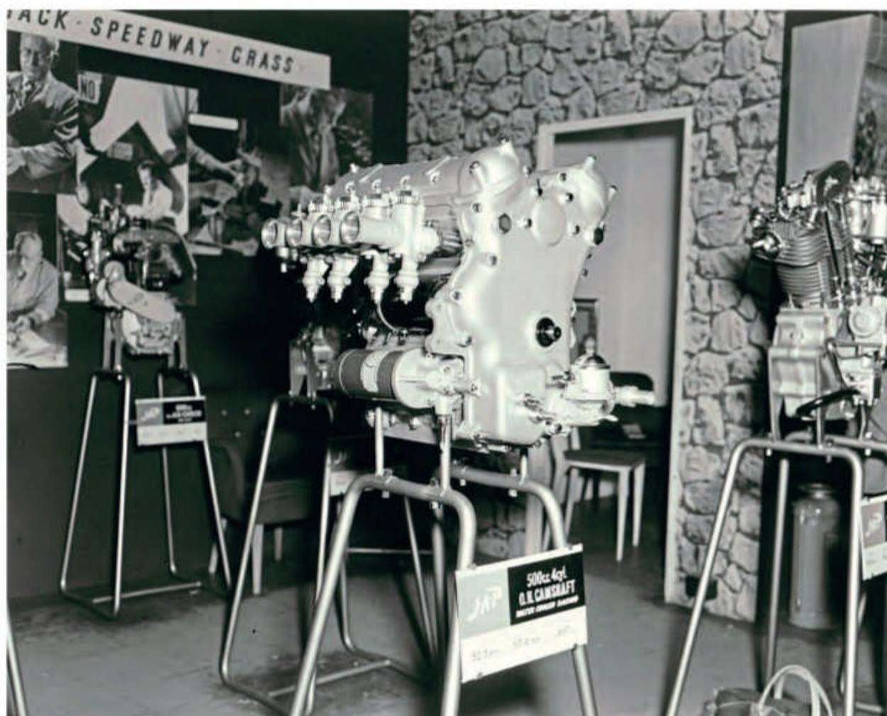
The Joe Rolando designed four cylinder engine - now, one wonders, how would that have performed in a Featherbed frame?
