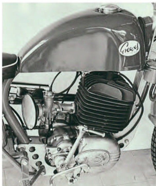
From 1966, Anglian Villiers engine with Challenger barrel and head.
