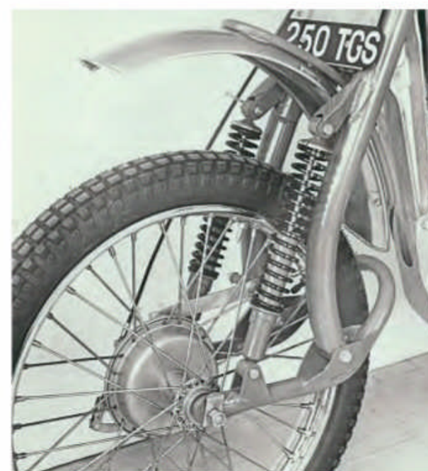
The 'banana' front fork fitted to all Anglians (1966-8) as standard, though teles were available for another £20.
