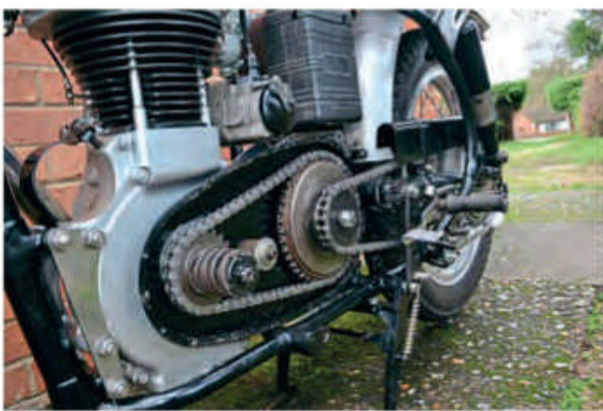
Chains, both primary and final drive, are new too.
