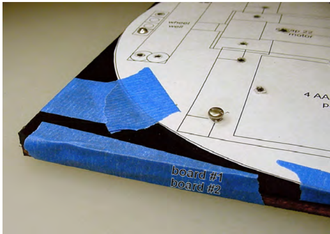
Figure 13-16. Two boards and a paper template originally held together with low-adhesive tape. After drilling and tapping, screws hold the boards together so that tape is no longer necessary. You should then remove the tape before machining the outer edges.
