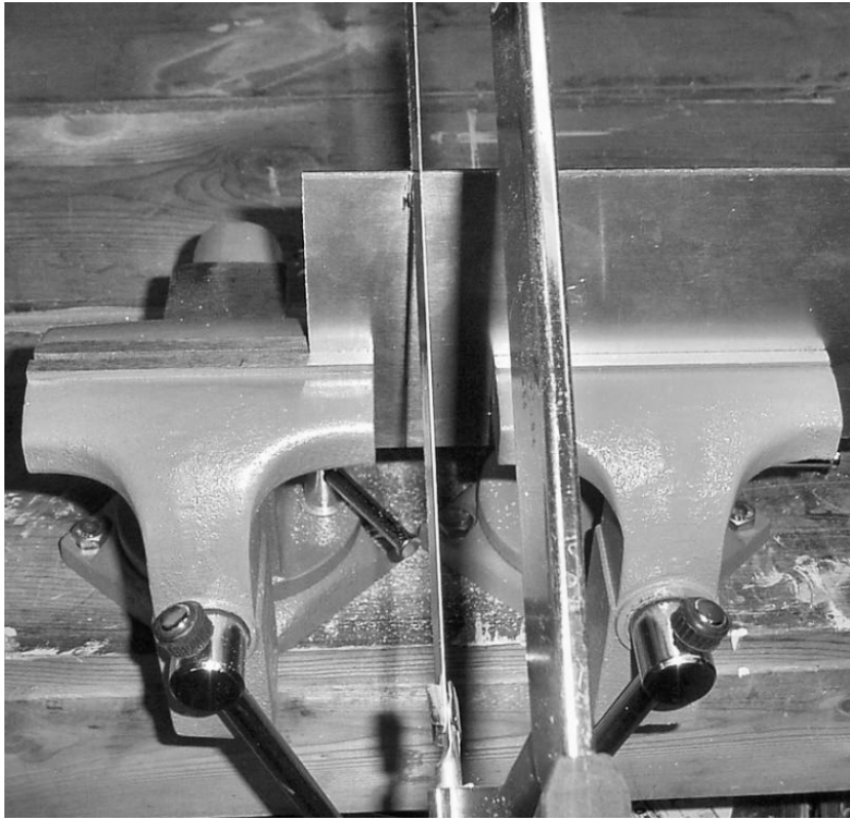
Figure 5-7. Aluminum sheet held between two bench vices while being cut by a hacksaw
