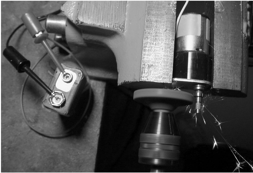
Figure 18-19. Grinding down the wide portion of the shaft with a Dremel grinding stone accessory. The gearmotor is powered by a rechargeable 9 V battery (about 7.2 V) to rotate the motor shaft during grinding to ensure the reduction is even all the way around. The grinding process produces spectacular sparks.
