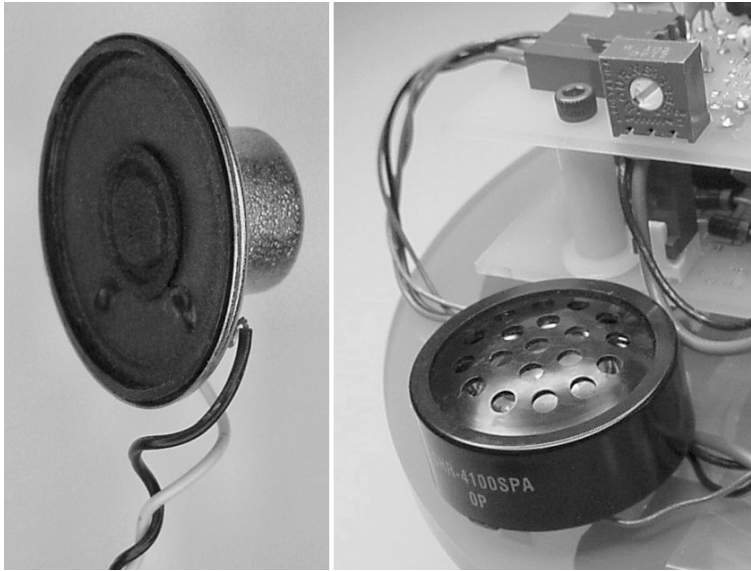
Figure 18-2. An ordinary 8\Omega speaker removed from a discarded personal computer (left). A compact speaker with protective cover that's glued to a piece of plastic and screwed in from underneath (right). Note the square trimpot (R5) at the top right of the picture, which adjusts the volume.
