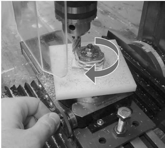
Figure 5-13. The mill slowly approaches the center of the rotary table as you turn the handwheel to cut the stock evenly on all sides.
