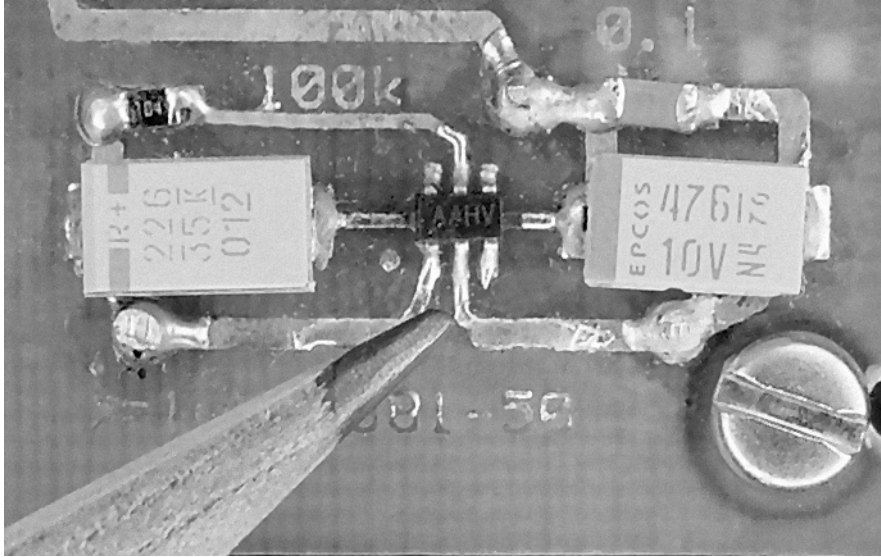
Figure 7-14. The Maxim ( http://www.maxim-ic.com/ ) MAX8881EUT50 is a 200 mA maximum load, low-dropout, 5 V linear voltage regulator with a maximum quiescent current of only 3.7 \mu A. The regulator circuit for the MAX8881 is as simple as those presented in this chapter. However, this regulator isn't easy to prototype on a solderless breadboard because the chip is as small as the head of a pencil. The size comes in handy for size-constrained robots, such as a mini-sumo robot. This picture is from the circuit board of the mini-sumo robot Have a Nice Day .
