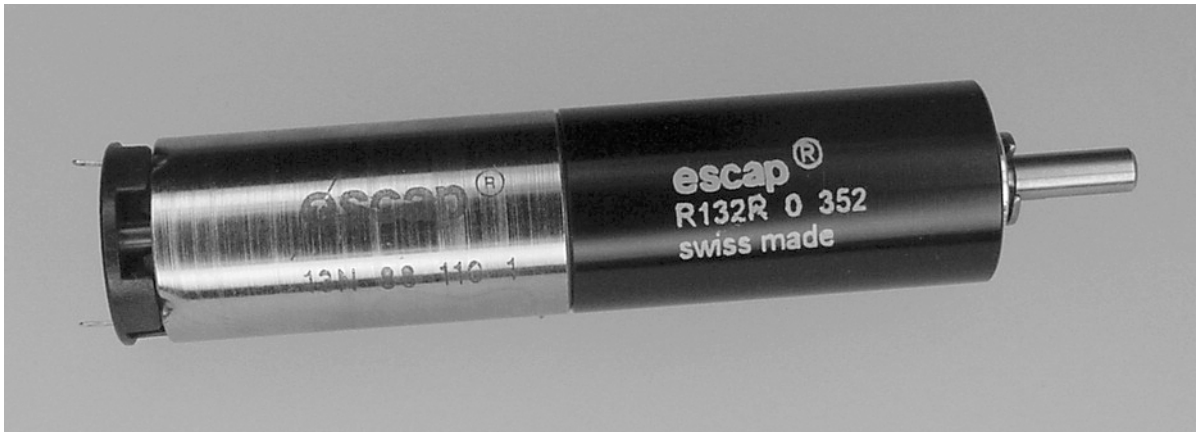
Figure 13-11. Small-diameter Escap motors drive Roundabout.
