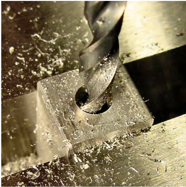
Figure 3-19. Drilling the coupler rod hole
