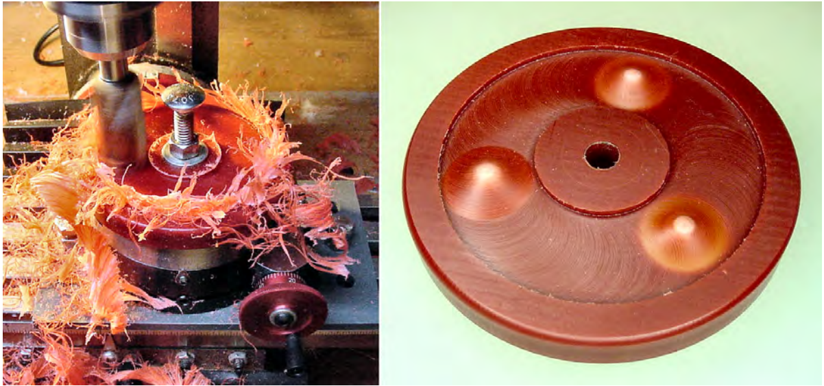
Figure 5-18. Creating depth by milling away some disc material while mounted on the rotary table (left). Partially drilling three holes from the opposite side resulted in the plastic melting and deforming to match the contour of the drill point (right).
