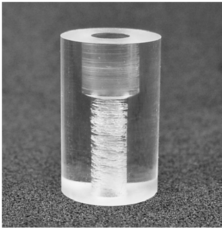
Figure 2-4. Desirable: Coupler with nicely centered, straight-angled holes
