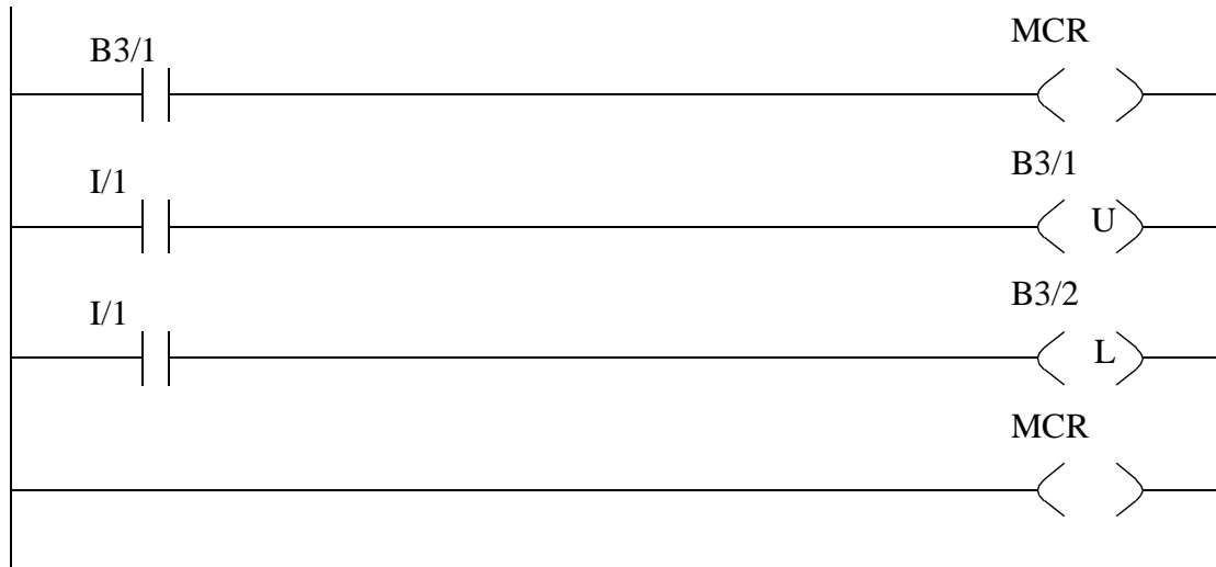
Figure 12.12 Ladder Logic for First State
