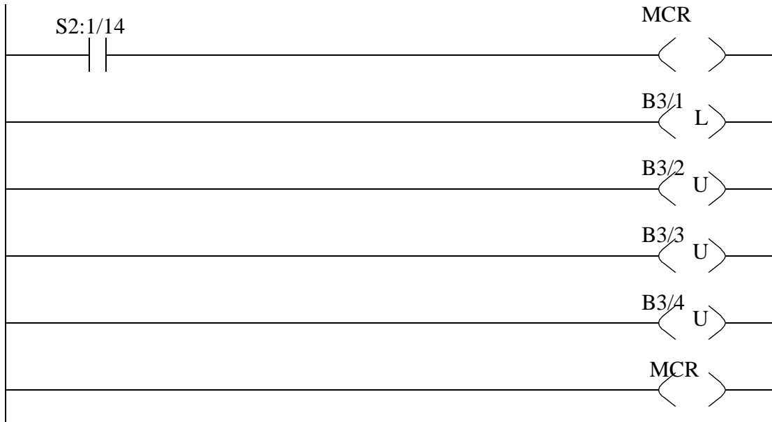
Figure 12.10 Ladder Logic to Initialize Traffic Light Controller
