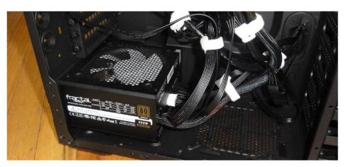
components. A modular PSU's cables are all detachable, meaning you can connect just the cables you need and avoid a tangle of unused cables in your PC case. A semi-modular PSU has only the essential power cables attached, with the rest of the cables detached until you need them. A non-modular PSU arrives with all its cables already attached, so no need about worrying whether you've got all the power cords you need.
