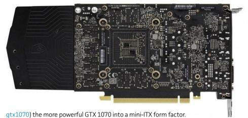
Also like the Radeon RX 480, the GTX 1060's a full-length dual-slot graphics card despite its shrunken PCB. The final quarter of the card is pure fan and shroud—almost. Interestingly enough, Nvidia still slapped the 6-pin power connector on the end of the card's edge, and not on
