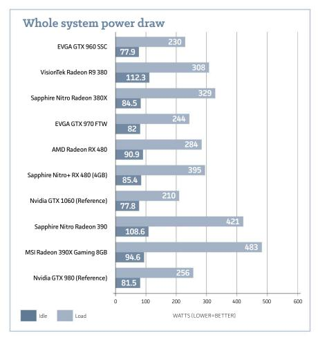
slightly more power than the reference RX 480 under load. But that Dual-X cooler helps out when you're not playing games, as the Nitro+ RX 480 consumes a bit less power than its reference cousin at idle.
