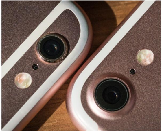
Bigger is better. The f1.8 aperture lens on the back of the iPhone 7 (right) takes much better photos in low light than the iPhone 6s.
