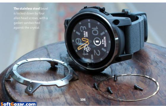
My review specimen came with a brushed stainless steel bezel, but when you order the watch, you can choose from 12 different bezel looks—five brushed steel options, and seven matte cerakote (go. pcworld.com/cerakote) options. The bezel is held down by four easily removed allen-head screws, but there's really no reason to disassemble the watch, as Nixon isn't selling the bezels as standalone items for customization
