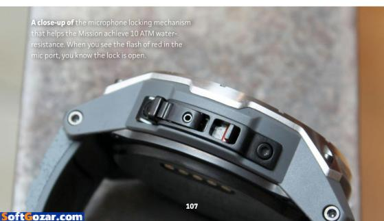
water in the shower But Nixon wanted a watch that could survive wipeouts and turtle rolls. Enter Nixon's MicLock mechanism, which helps the Mission achieve a 10 ATM rating. In theory, this means the watch can survive submersion under 330 feet of water
