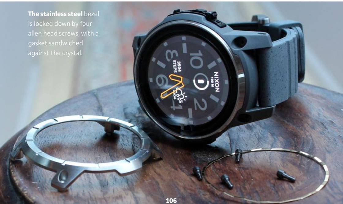
**The stainless steel** bezel is locked down by four allen head screws, with a gasket sandwiched against the crystal.
