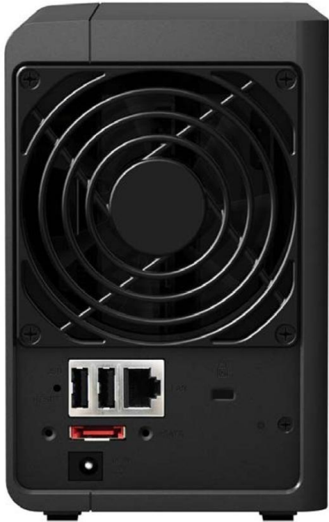
The inclusion of an eSATA port on the DS216+ is a bit old-school for a modern SOHO NAS box.
