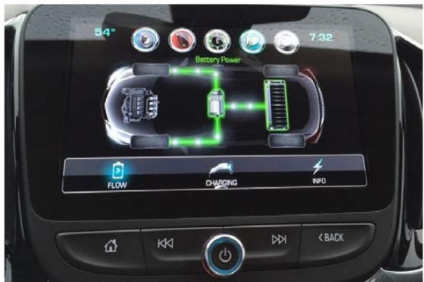
The 8-inch center touchscreen on the 2016 Chevy Volt offers, among other views, an animated illustration of the gas and electric power distribution as you drive.
