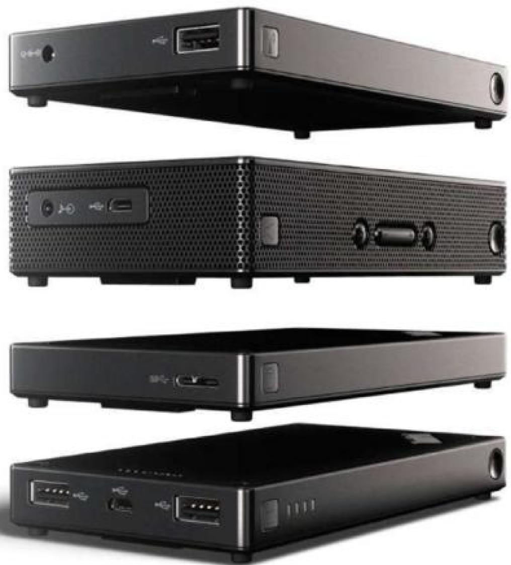
a personal Wi-Fi network (an 802.11ac router), powering the stack and charging your devices (a battery), and making noise (a Bluetooth speaker).
