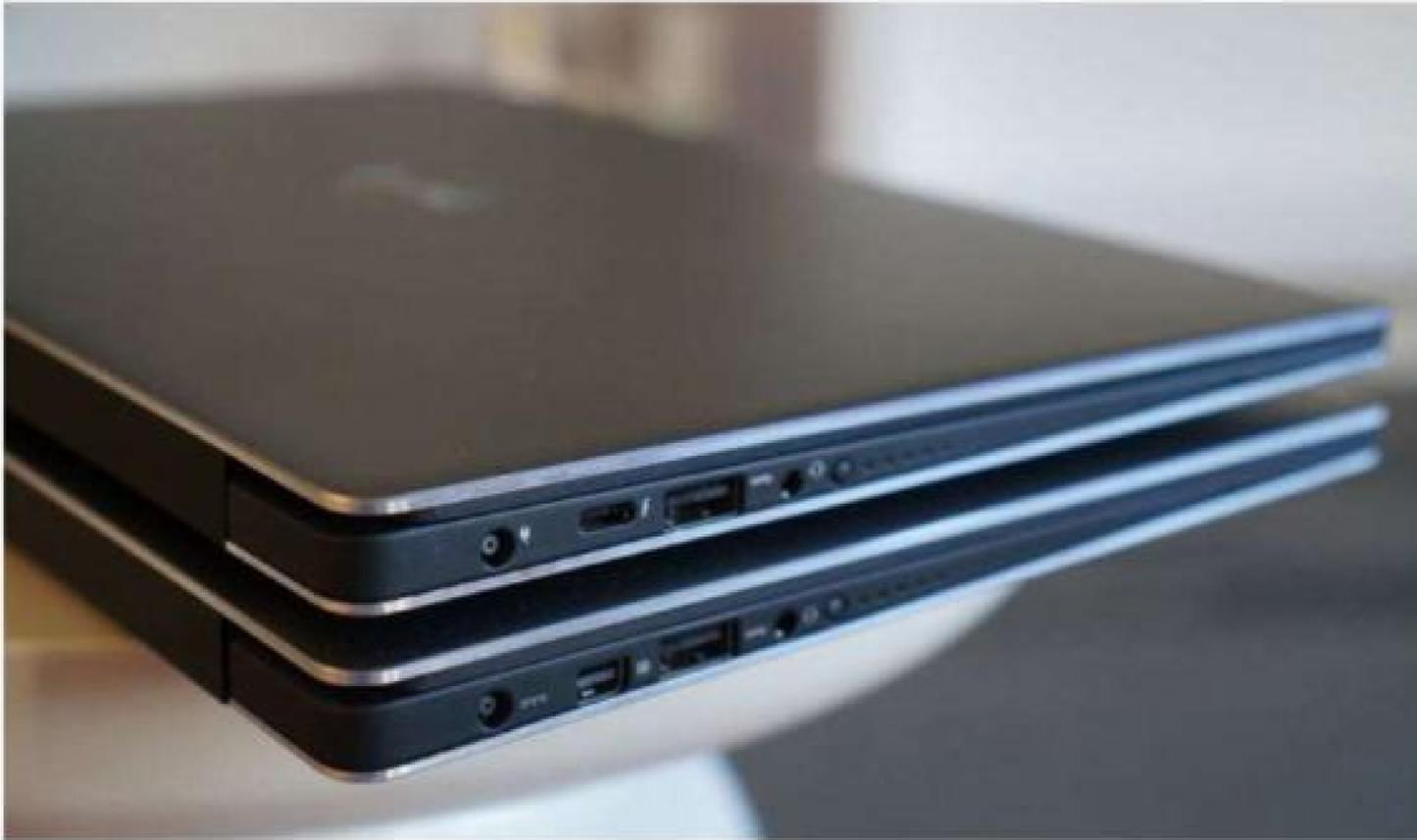
**The 2016 XPS 13** on top of the 2015 model. The only real external difference you can see is the move from mini DisplayPort to USB-C.
