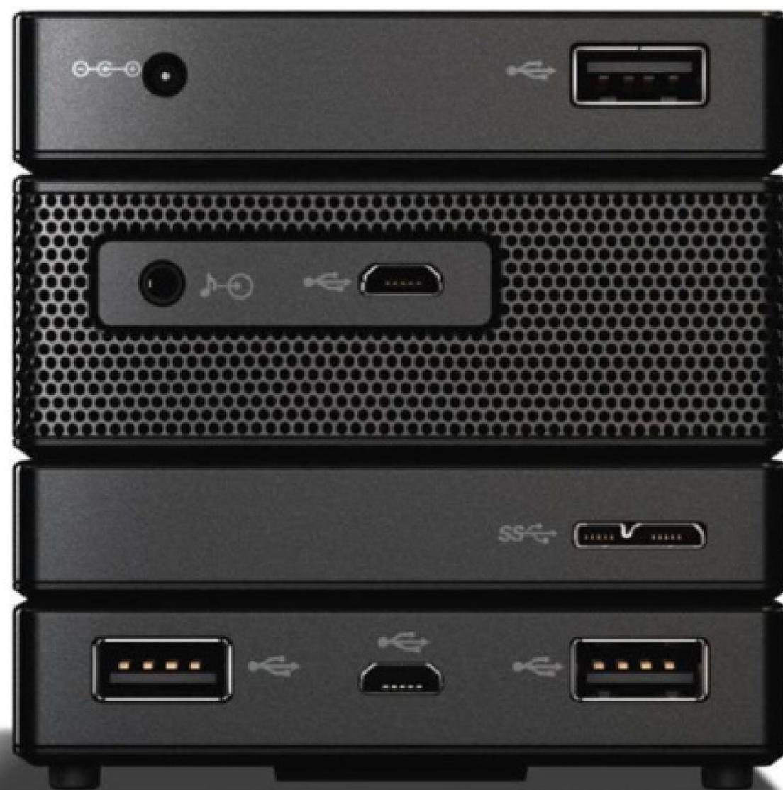
**The side of** the Stack with all of the ports, except, for some reason, the Ethernet port, which is located on another side, 90 degrees away.
