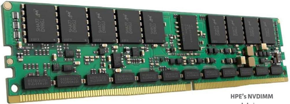
**HPE's NVDIMM module** has DRAM chips and multiplexors on the front, connected to NAND flash chips on the back.
