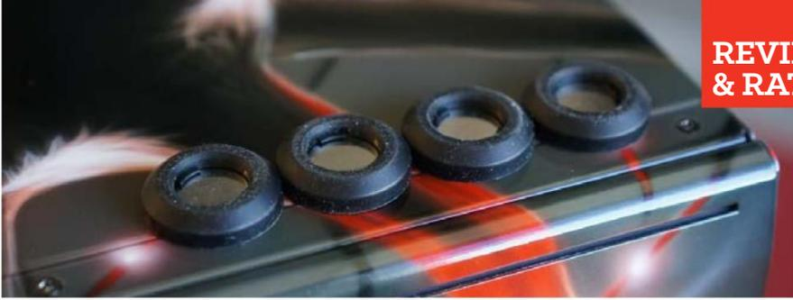
**They're just magnets**, but the removable feet work relatively well and can be moved depending on the orientation of the case.
