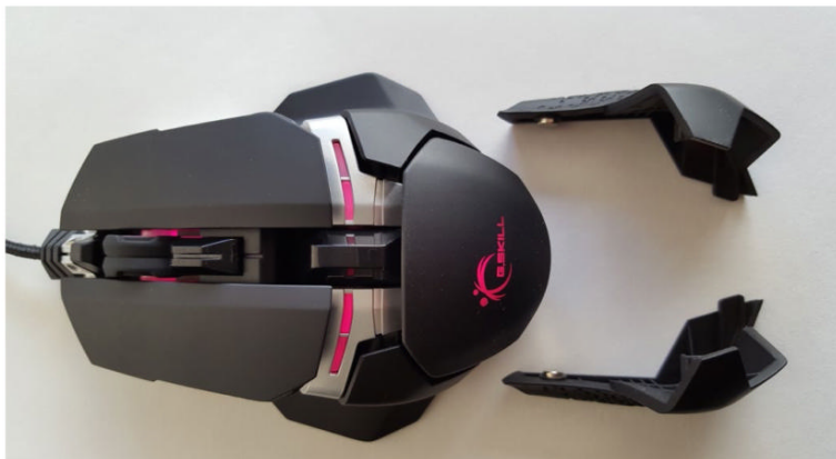
Mouse customization channels are held in place with magnets.
