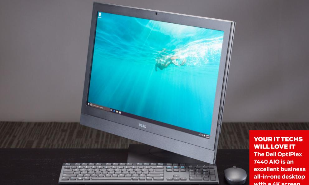
angle (about 30 degrees), and it allows you to swivel the monitor and switch between Landscape and Portrait modes. Our review unit also shipped with a chiclet-style wired keyboard and wired mouse, which both performed smoothly; a wireless keyboard and mouse set is optional.
