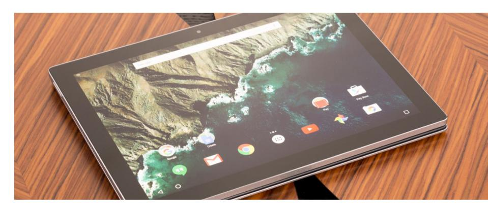
The Pixel C's 10.2-inch LCD has a 2,560-by-1,800-pixel resolution for a peculiar (but benign) aspect ratio of the square root of two. Colors are rich if you're looking at the screen face on, and they look natural rather than oversaturated the way they can on many OLED screens. On the other hand, I found the display to be distractingly reflective when the tablet is laid flat on a table.
