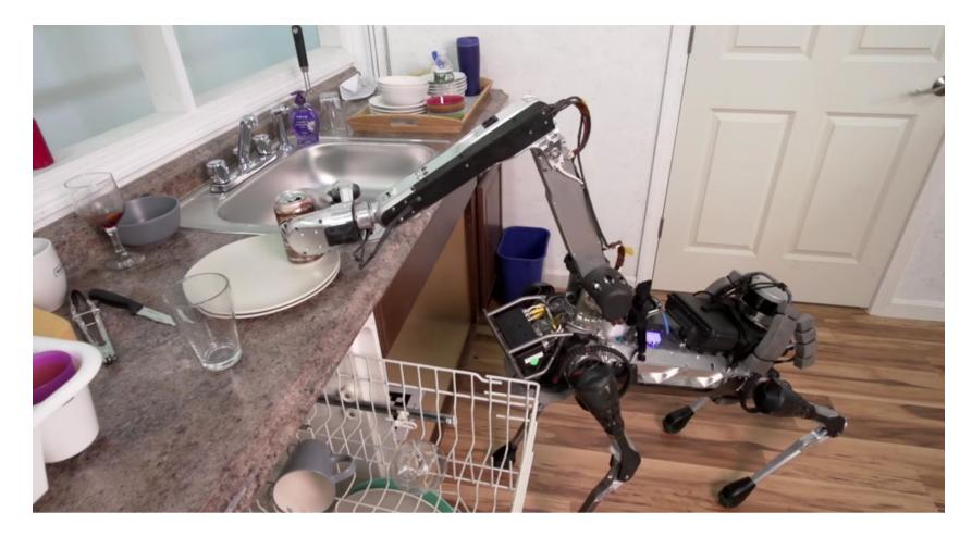
At 1:01, we see SpotMini carefully loading glasses into a dishwasher. When it encounters an A&W Root Beer can, it picks the can up and deposits it into a recycling container. Less clear is whether Robo Dogmeat can perform this task when confronted with containers that blur the line between an obvious recyclable (aluminum can) and objects more likely to be reused—plastic water bottles, glass bottles, mason jars, and other types of containers. Still, this is significant progress.
