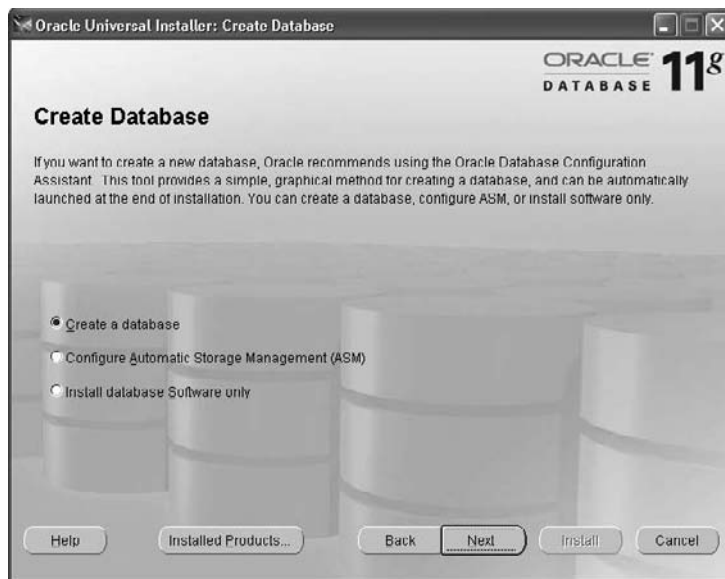
FIGURE 3-2. Choose to install ASM in Oracle Database 11g R1 or earlier versions
