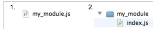
Figure 3.3 Node modules can be created by using either files (example 1) or directories (example 2).
