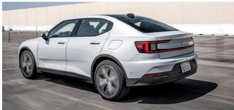
As of now, all Polestar 2s are equipped with front and rear motors with a total system output of 402 hp and 487 lb-ft of torque. Due to the permanent-magnet nature of the motors—meaning they must always be driven and can't freewheel—the Polestar 2's range pales in comparison to the rival Tesla Model 3, which nets 141 mpg-e combined and 250 miles of range on the EPA cycle to the Polestar's 92 mpg-e and 233 miles of range. And for 2021, Tesla is promising 263 miles of range on a base Model 3.
