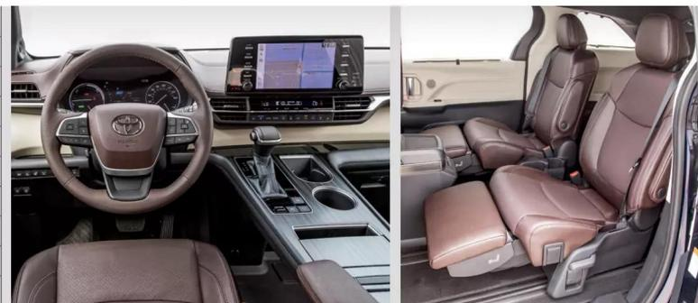
**VEHICLE LAYOUT** Front-engine, FWD, 7-pass, 4-door van **ENGINE/TRANSMISSION** 2.5L Atkinson-cycle DOHC 16-valve I-4/Cont variable auto **CURB WEIGHT (F/R DIST)** 4,714 lb (55/45%) **WHEELBASE** 120.5 in **LENGTH x WIDTH x HEIGHT** 203.5 x 78.5 x 68.5 in **ENERGY CONS, CITY/HWY** 94/94 kWh/100 miles **CO2 EMISSIONS, COMB** 0.54 lb/mile
