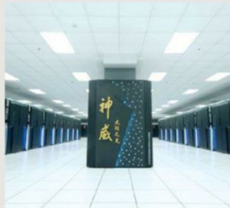
China's TaihuLight has 40,960 nodes, with 260 cores per node.
