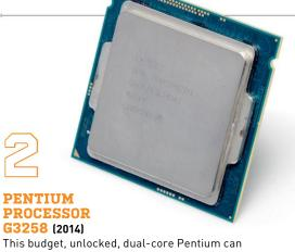
hit 4.5GHz from its 3.2GHz base, making for a great starting point for any LGA1150 system.
