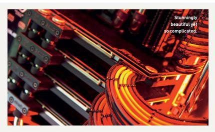
more cooling potential), you can move that heat away from your components far faster, and dump it into the radiators far quicker, than with air cooling. Couple that with the astronomical level of surface area available in a 240mm rad compared with an air-cooled tower, and we're on to a winner. Then, of course, there's the
