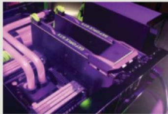
**Pascal modifies Nvidia's SLI to support a new HB connector for improved two-way SLI capability.**
