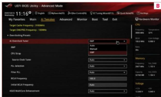
higher multiplier. So, if you have a Core i7-6700K reading “42,” input “44.” Hit F10, save, and reboot, then head to the desktop to see if it’s stable. At this point, it’s not worth messing with voltages.
