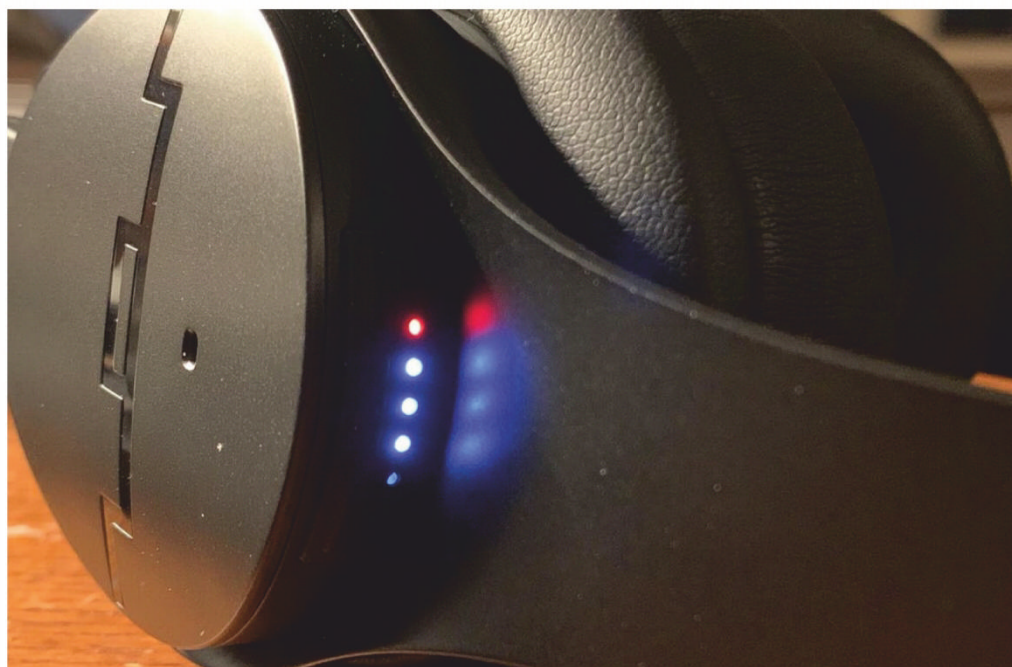
Lights on the top of the right earcup let you know the charging status.
