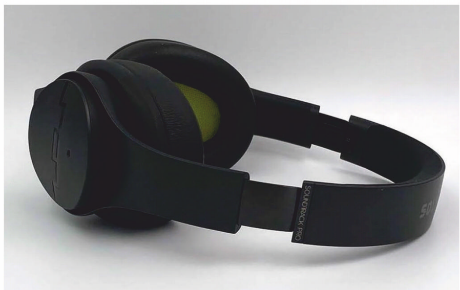
The SOL Republic headphones are mostly plastic with the click-adjustable headband a noticeable exception.
