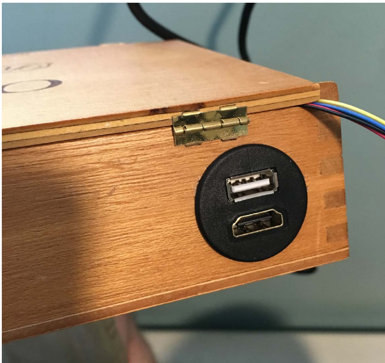
Figure 10. Another cheat: the HDMI/USB flush-mount extension required me to drill a big round hole instead of chipping out a square mounting hole.
