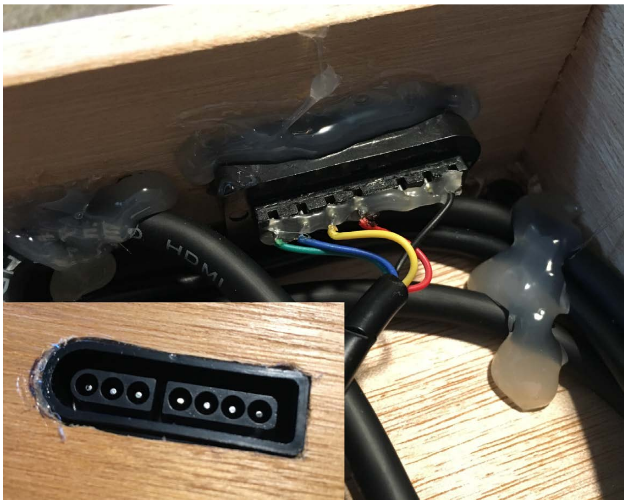
Figure 6. The mounting holes are ugly, but hot glue covers a multitude of sins.
