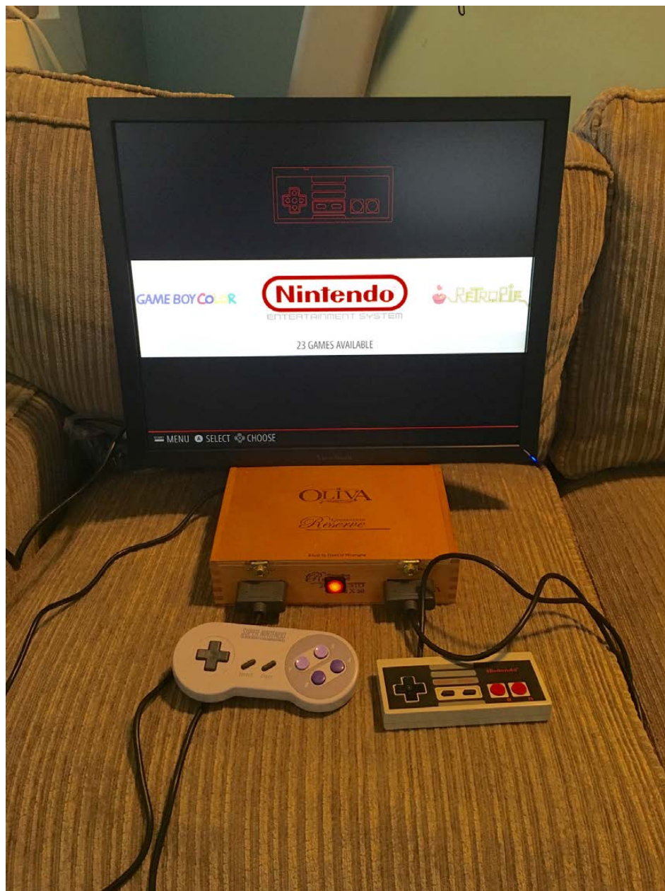
Figure 1. This is the completed system. Notice the working power LED and both types of controllers plugged in. The screen shows Emulation Station's front end.
