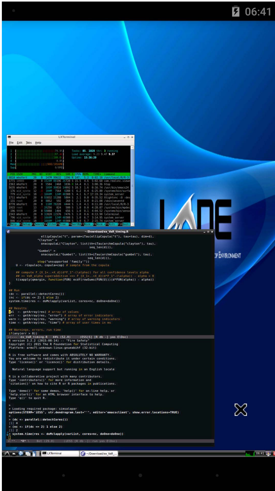
Figure 7. R Code Running on Two Cores of a Google Nexus 5 Android Smartphone over a VNC Connection via VNC Viewer
