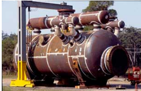
Figure 2: Forced Circulation Crystallizer (Horizontal Heat Exchanger)
