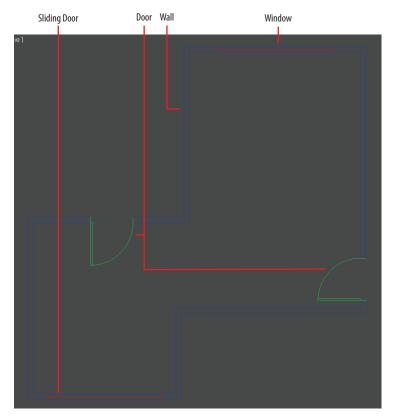
FIGURE 3.5 An AutoCAD drawing showing walls, doors, and window
