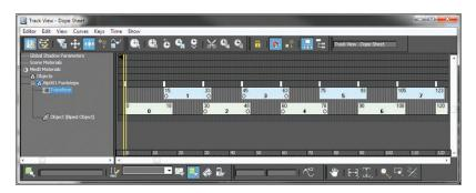
**FIGURE 13.10** The dots indicate when contact begins and ends. You can drag a dot to change the duration of contact.
