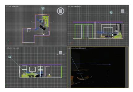
**FIGURE 16.30** Move the Daylight System light so it will shine through the window.
