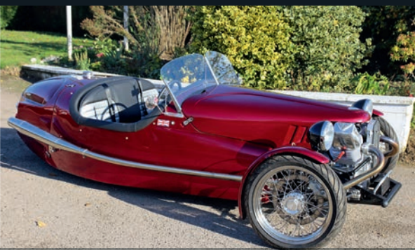
Typically, this 360kg three-wheeler has a 120bhp Moto Guzzi unit
