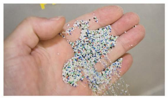
▲ STEP 2 Plastic media consists of small plastic beads applied at force to the surface to be stripped. They are softer than most other compounds used in blasting and are applied at a much lower pressure. As a result, they don't cause panel buckling or other damage sometimes associated with other stripping methods.
