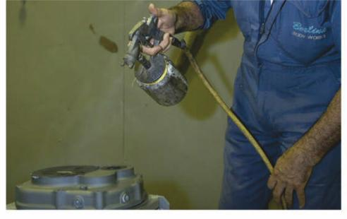
ightharpoonup STEP 9 Most parts are finished with a metal prep coat to prevent stripped surfaces from rusting.
