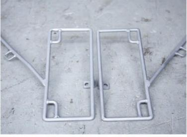
These stripped pannier rails won't be prepped as they're heading out to be powder coated; the prep coat would interfere with that process.
