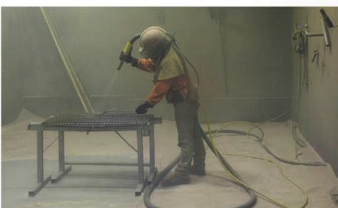
▲ **STEP 7** The pannier racks are now placed in the garnet blasting room where they are whipped, particularly in areas where surface rust is evident.
