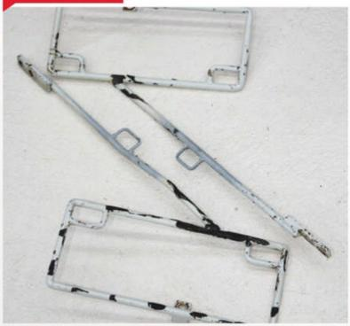
▲ **STEP 1** Parts like this need to be stripped of all old paint and surface rust before being refinished with paint or other coatings.
