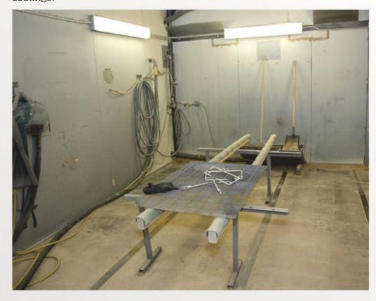
▲ **STEP 3** The part is placed in a sealed blasting room. The process is dry and environmentally friendly (all residue is bagged and recycled).
