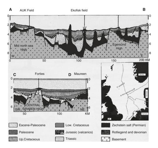
Fig. 14.5 Geological profiles under the North Sea, with hydrocarbon fields. Vertical exaggeration 6.7×. *Insert*: Map with national shelf boundaries (After P.A. Ziegler, 1977, modified for clarity. See *Geol. Journal* 1:7)
