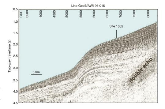
Fig. 3.6 Sediment stack off Namibia, southwestern Africa, explored with a small air gun in preparation of ODP Leg 175 (Seismic record courtesy of Volkhard Spiess, Bremen; color here added)
