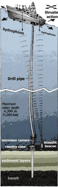
**Fig. 12.5** Retrieving information on Cenozoic history from the seafloor. The chief source of information is drilling from a vessel (here: the JOIDES Resolution is a vessel originally used by BP in commercial
