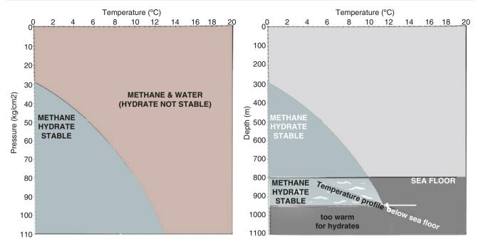
**Fig. 4.5** Stability field of methane ice (*left panel*, **a**) and application to sedimentary deposits (*right panel*, **b**). A bottom-simulating reflector (BSR) can occur at the bottom of the layer bearing methane hydrate. At the BSR sound is strongly reflected. The distribution of clathrate is restricted; its presence requires appropriate temperature and pressure to ensure survival if clathrate is present, in addition to a source of methane
