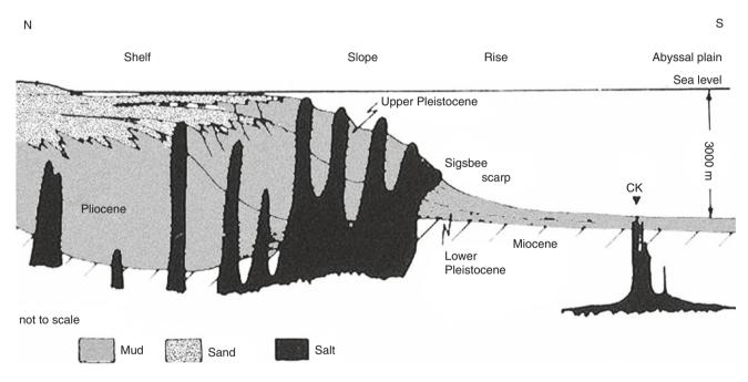
Fig. 14.4 Salt plumes in the Gulf of Mexico: Mesozoic salt intruding Neogene mud (After C.J. Stuart and C.A. Caughey, 1977, AAPG Geol. Mem., 26, modif.; "CK", Challenger Knoll, a salt dome below the continental slope (position from DSDP Leg 1))
