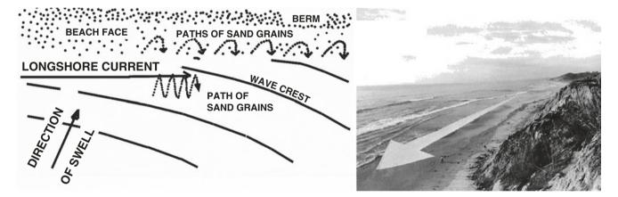
**Fig. 5.7** Sand motions on the beach. Overall, sand moves southward on both West and East Coast of North America, driven by waves from northern storms (Graph and image inspired by W. Bascom (*graph on*
