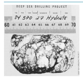
**Fig. 12.16** Methane ice (methane clathrate) embedded in black mud (DSDP Leg 84; photograph from S.I.O. archives)
