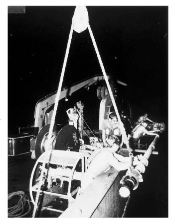
**Fig. 11.1** Recovering the Pleistocene record by piston coring. The corer is a wide-diameter model; note the white sediment in the core nose. Other equipment seen on deck: deep-sea camera frame (with protective grid), hydrophone for seismic profiling (wrapped on a spool), and box corer (aft) (SIO Eurydice Expedition, 1975; photo Tom Walsh; taken at night)
