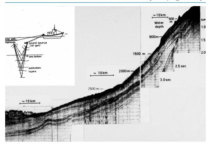
**Fig. 3.14** Submarine mass movements off Dakar (Senegal, NW Africa). Air gun record of Meteor Cruise 25/1971. Thickness of slide is ca. 200 m. (Note vertical exaggeration.) *Insert*: air gun system with air
