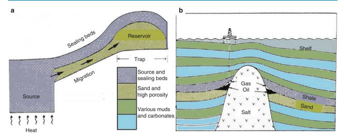
Fig. 14.3 Schematics on hydrocarbon accumulation. (a) Basic elements of a petroleum reservoir system, with migration from heated source rocks to a porous reservoir. (b) Offshore salt dome tectonics generating trapping conditions
