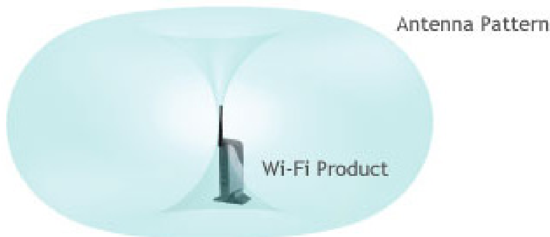
Figure 1. Knowing what the signal looks like helps with placement (image from http://ampedwireless.com ).
