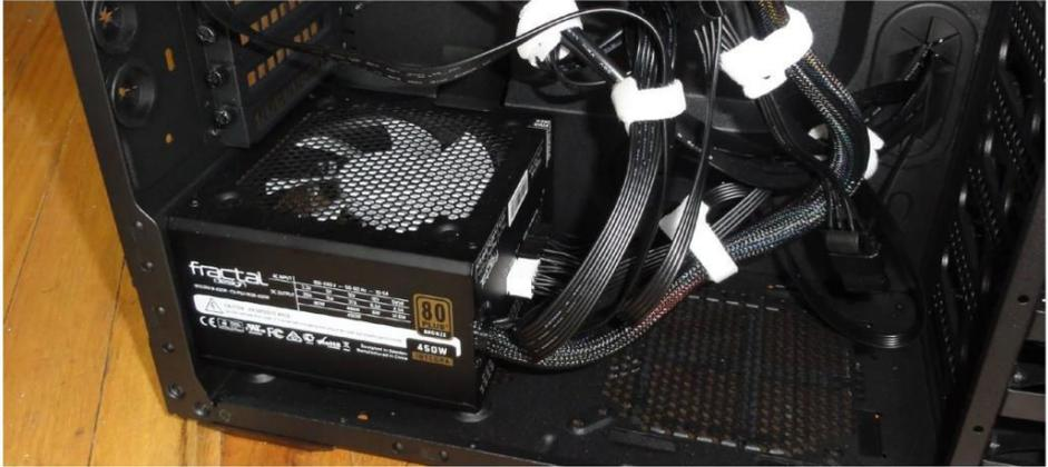
components. A modular PSU's cables are all detachable, meaning you can connect just the cables you need and avoid a tangle of unused cables in your PC case. A semi-modular PSU has only the essential power cables attached, with the rest of the cables detached until you need them. A non-modular PSU arrives with all its cables already attached, so no need about worrying whether you've got all the power cords you need.
