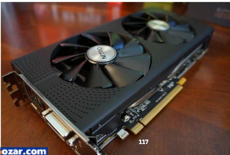
**The Nitro+ RX 480** features Sapphire's superb Dual-X cooling solution, with easily removable fans.
