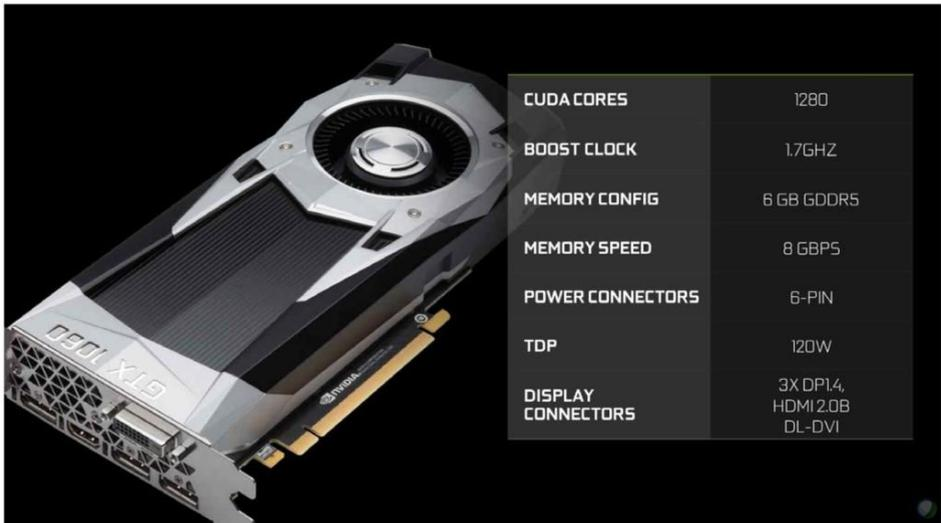
6GB of GDDR5 memory clocked at 8Gbps. Nvidia’s new card sports the same HDMI 2.0b port and trio of DisplayPort 1.4 connections as the other GTX 10-series GPUs to ensure compatibility with VR headsets and ultra-high resolutions alike, along with a DVI-D (not DVI-I [go.pcworld.com/ripvganvidia](http://go.pcworld.com/ripvganvidia)) port for lower cost displays.
