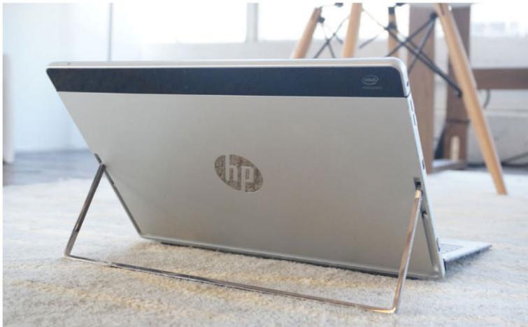
**Here's a full view** of the kickstand design HP uses on its Surface clone.
