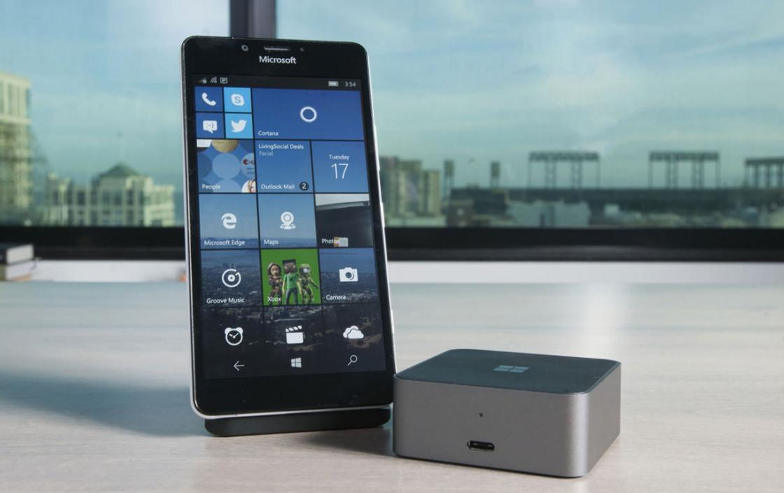
Continuum can connect your phone to an external display with or without wires, but it works best with the \$99 Microsoft Display Dock, which connects to—and powers—either the Lumia 950 or 950XL via its USB-C cable. (The Display Dock does not have a Micro-USB input, such as that used by older Windows Phones.)
