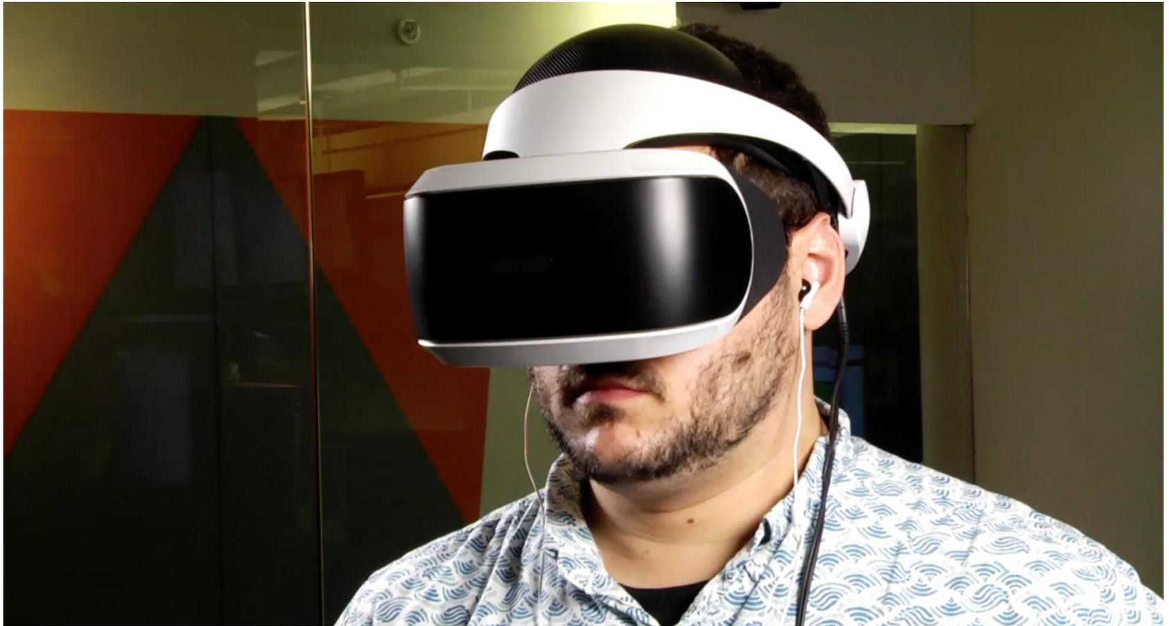
PlayStation Camera to track the headset's location. A wire runs from the left side of the visor and partly along the headband before dropping down to connect to the PS VR processor box with the included cable.
