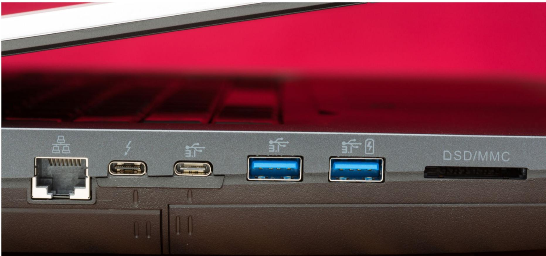
As mentioned, the port inclusions are different this time around, with a lot of variety offered. On the left side are two USB 3.0 ports and two USB-C ports—one with Thunderbolt 3. You'll also find an Ethernet jack and an SD card slot. On the right flank are two more USB 3.0 ports and four audio lines for microphone,
