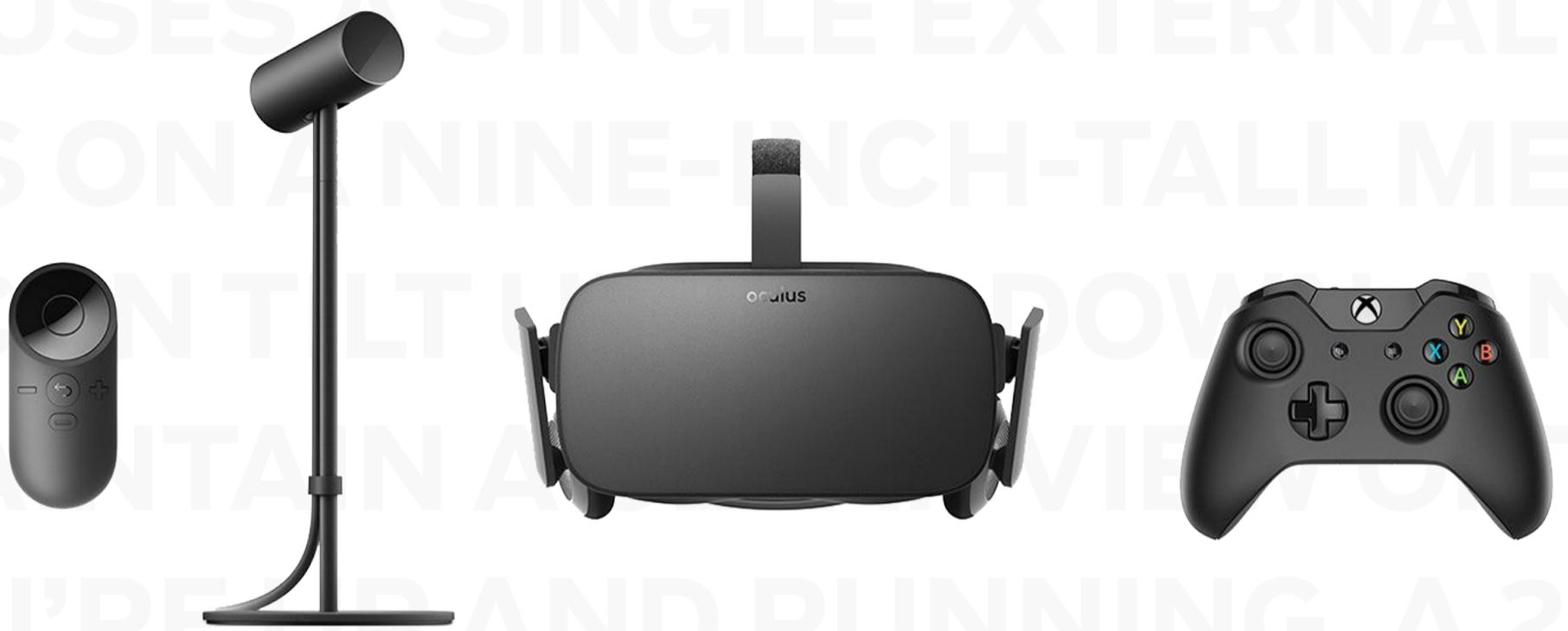
Oculus plans to offer Touch motion controllers separately later this year, but the headset still comes with some control options, including the Oculus Remote. It's a small, rounded remote control with a large, circular navigation pad and Back, Menu, and Up/Down buttons. The remote helpfully features a lanyard to keep it attached to your wrist when you're using the Rift. In the box you also get a Microsoft Xbox One wireless gamepad, along with a wireless receiver for the gamepad.
