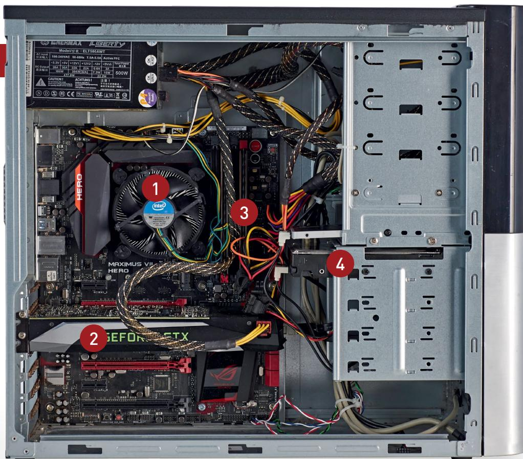
**1 CPU** Ultimately, we decided to forego upgrading the processor. The Intel Core i5-4670K inside this machine holds more than enough potential to handle any game or program we can throw at it. And if we really need to, we can swap out the cooler for something chunkier, and crank those hertz up.
