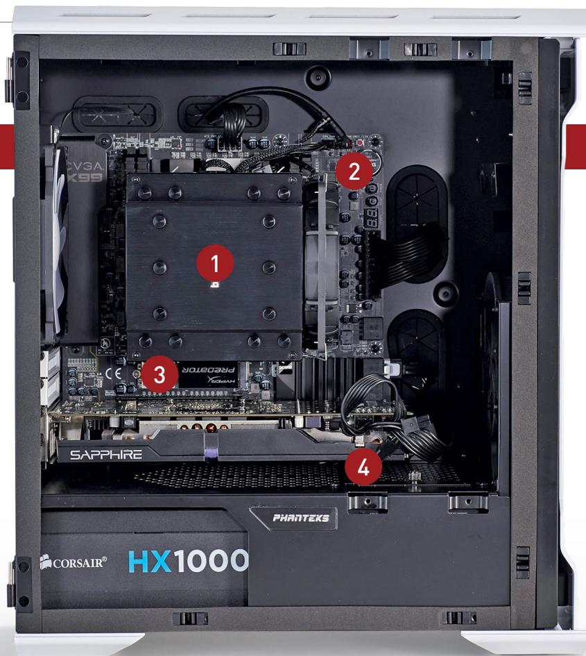
**1 CPU** The CPU was the second-biggest change we made to this system. Jumping forward by five generations of processor technology has helped to push performance up by almost 35 percent in contrast to the Intel Core i7-970 that was originally found in this machine. A very worthwhile upgrade.
