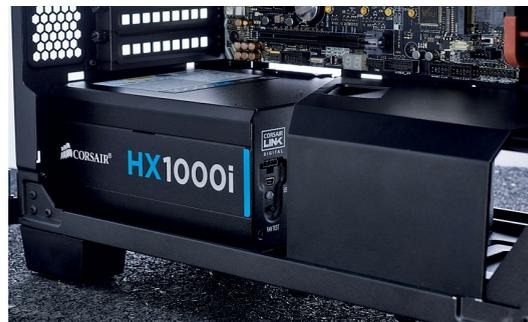
our new upgraded system (including older GPUs and hard drives), which provided us with a good estimate of what our overall power usage was going to be (471W at peak). You should always look for a power supply that provides somewhere in the region of 20–25 percent more rated power than your system draws from the wall. That way, you'll never run it at max capacity, and PSUs are generally most efficient when they run at 80–90 percent capacity.
