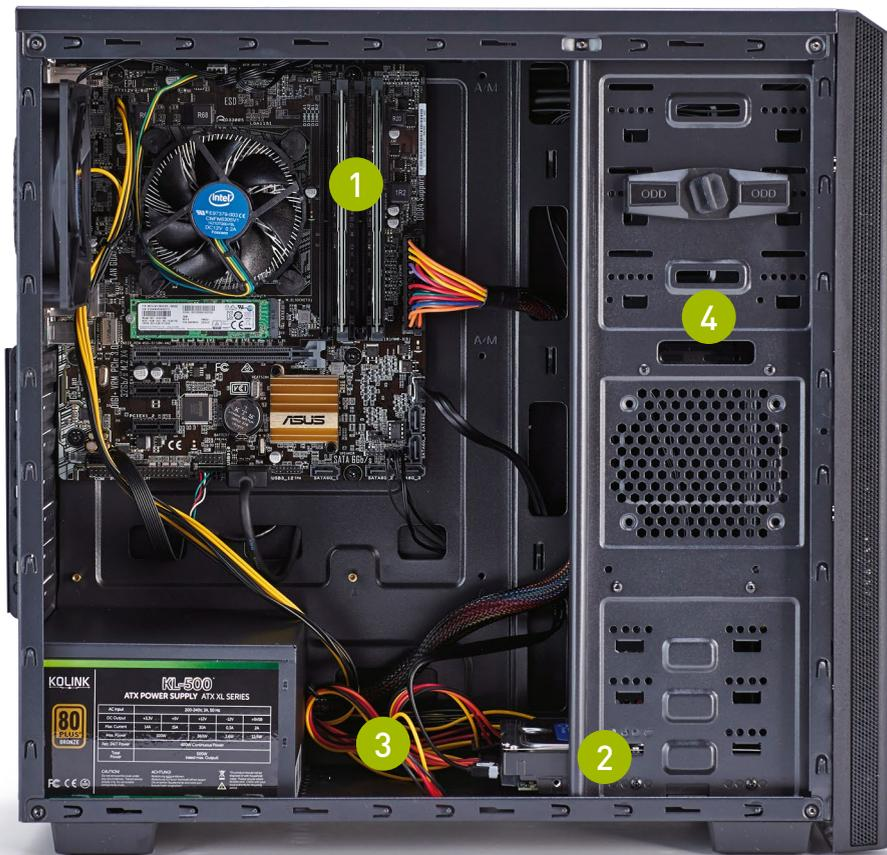
**1** The 8GB of DDR4 here is rated to operate at 2,400MT/s—it's worth noting that the B150 chipset can only support 2,133MT/s max.
