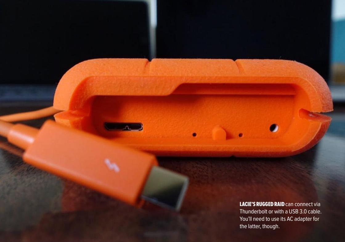
**LACIE'S RUGGED RAID** can connect via Thunderbolt or with a USB 3.0 cable. You'll need to use its AC adapter for the latter, though.
