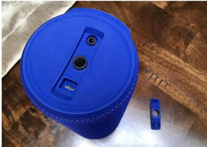
**REMOVING THE GASKET** on the Megaboom's bottom reveals the micro USB charging port and 3.5mm analog input.
