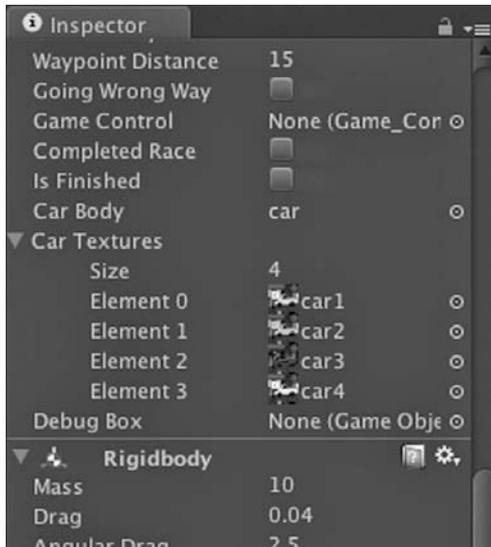
**Figure 6.7.** The car textures populating an array in the Inspector window of the Unity editor.
